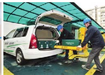
Figure 14: Rear battery mount
