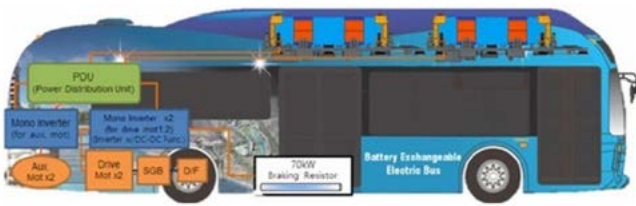
Figure 9: Battery-swapping positioning on a bus. Source: Kim et al., 2015.
