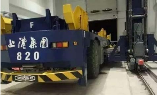
Figure 34: AGV battery-swapping solution at Yangshan Port, Shanghai.
