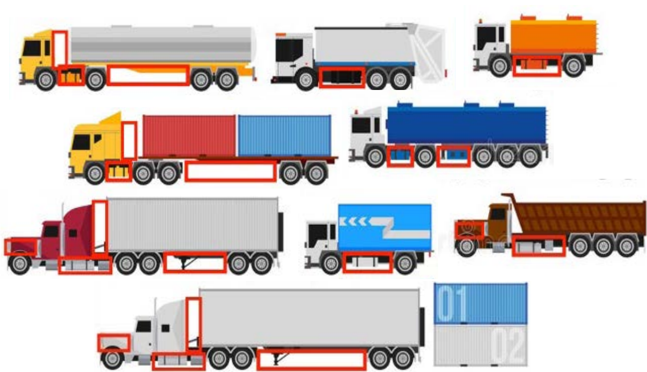
Figure 8: Battery-swapping positions on a truck.
