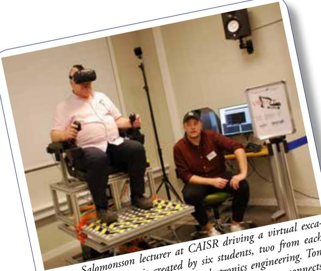
Tommy Salomonsson lecturer at CAISR driving a virtual excavator. The simulator is created by six students, two from each: computer-, electrotechnical- and mechatronics engineering. Tommy was their supervisor in the project. The simulator connects a virtual environment to a platform that moves and reacts according to the excavator work. Patrick Karlsson that worked with the gamification software is supervising the work.
