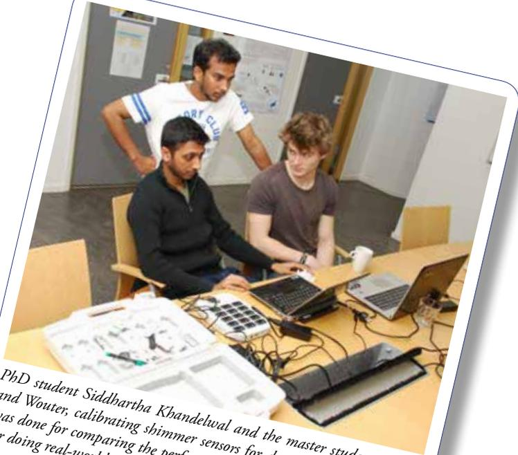
*PhD student Siddhartha Khandelwal and the master students Lobith and Wouter, calibrating shimmer sensors for data collection. The work was done for comparing the performance of accelerometers vs gyroscopes for doing real-world gait analysis.*
